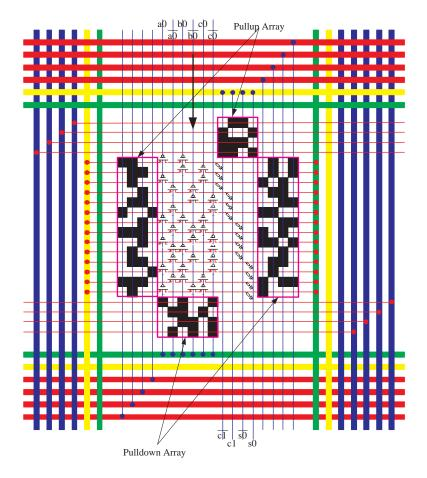
Figure 3: Optimized 1-bit adder realized with NOR-OR NW logic.
