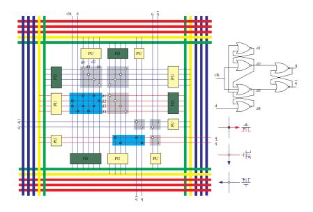
Figure 4: 1-bit Flip-flop design with NWs.
