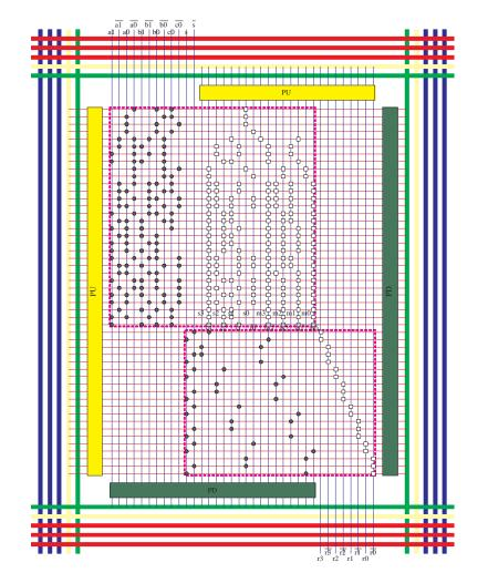
Figure 6: A simple stream-processor realized with NW FETs. The processor demonstrates the capability of selecting between a multiplier and an adder with a control input. The adder and multiplier logic are combined. The design includes a multiplexer at the bottom of the figure.
