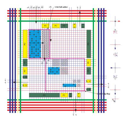
Figure 5: 1-bit data-path with NOR-OR NW logic.
