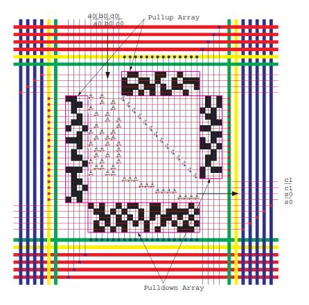
Figure 2: 1-bit adder realized with NW FETs.
