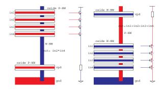
Figure 1: OR/AND logic implemented with SiNW FETs.
