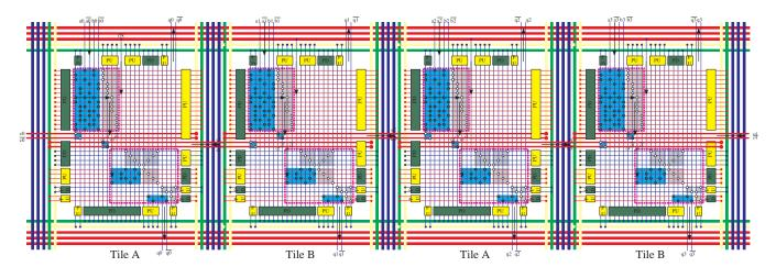
Figure 7: 4-bit adder realized with NW FETs in a 4-tile cascaded design. Two different tile types are necessary to achieve good fabric utilization.
