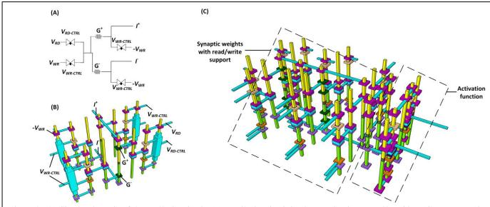
Figure 4. (A) Circuit schematic of the read/write circuit; (B) Read/write circuit implementation in Neuro-SkyBridge; (C) Perceptron in Neuro-SkyBridge.
