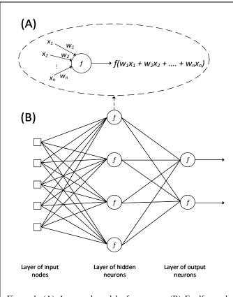
Figure 1. (A) A general model of a neuron; (B) Feedforward neural network
