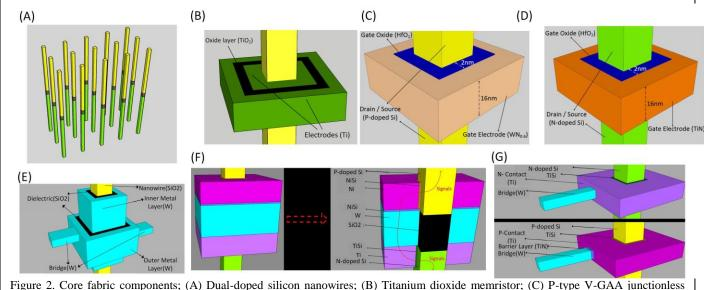
Figure 2. Core fabric components; (A) Dual-doped silicon nanowires; (B) Titanium dioxide memristor; (C) P-type V-GAA junctionless transistor; (D) N-type V-GAA junctionless transistor; (E) Co-axial routing structure; (F) SkyBridge-Interlayer-connection (SB-ILC); (G) Ohmic contact on n-type and p-type silicon with Tungsten bridges.
