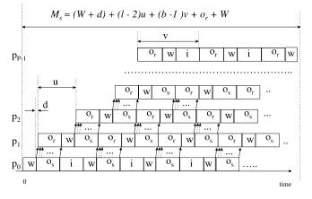
Fig. 8. A *Gantt chart* of computation and communication schedules for the Diamond DAG with stripe partitioning. The rectangular blocks represent the blocking send  $(o_s)$  and receive  $(o_r)$  overheads as well as computation times (w). The arrows represent communication between processors.
