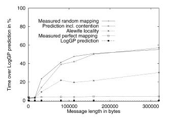
Fig. 9. Diamond DAG performance. Comparison of measured performance to model predictions with stripe partitioning, n = 1,024, b = 64, and each task takes 100 cycles. The "Alewife locality" curve uses the system default node numbering in the Alewife mesh. Node *i* sends to node i = 1, but numerically adjacent nodes are not always adjacent in the mesh.
