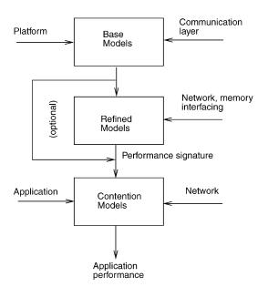
Fig. 1. An engineering perspective to performance modeling of parallel computer systems.
