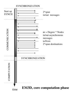
Fig. 10. EM3D core computation phase for E or H nodes.
