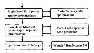
Figure 3. Experimental Setup Block Diagram
