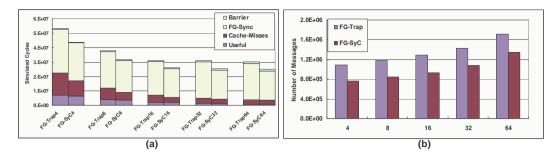
Fig. 7. (a) Execution time and (b) Number of messages of application DNA Chain under baseline (FG-Trap) and synchronization coherence (FG-SyC).
