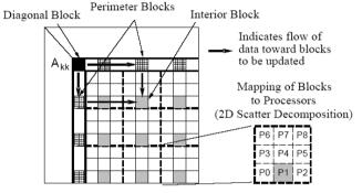
Fig. 6. LU factorization of blocked dense matrix [21].
