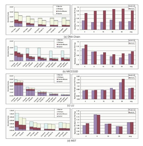
Fig. 17. Execution time of the applications with perfect L2 caches and speedup comparison with the case of no L2.
