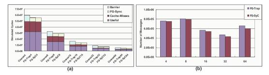
Fig. 9. (a) Execution time and (b) Number of messages of application LU under baseline (FG-Trap) and synchronization coherence (FG-SyC).
